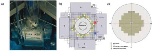
Figure 1. Schematics of the MINERVE reactor. (a) General view of the reactor [13]. (b) Schematic drawing of the MINERVE reactor structure [14]. (c) Schematic drawing of the MAESTRO core configuration [15]. The location of the IC and FC detectors is marked by red and blue circles, respectively, in panel (b).
